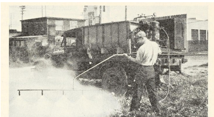
Fig. 7.—Power rig equipped with two lines—one air, one liquid—which produces atomization, thus giving a very even and thin coverage. This machine shows lines attached to multiple nozzle.
